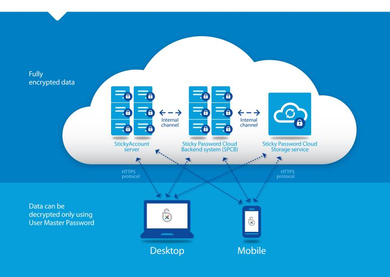
Figure 1: Sticky Password system architecture
